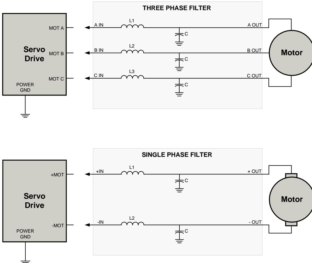
**NOTE: Capacitor is not used on all models. See Specifications above for applicable capacitance values**
